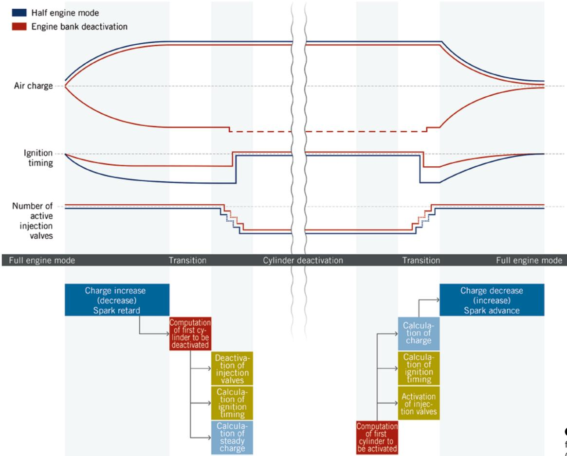
5 Transition control for cylinder deactivation (schematic view)
