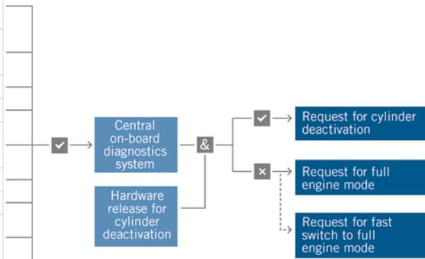
tioned quality criteria. The transition process begins by increasing the air charge so that the cylinders that are still activated can generate all of the required torque. In an engine with a single intake manifold, the increase is made across all
