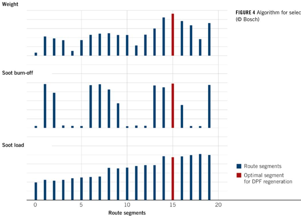
FIGURE 4 Algorithm for selecting regeneration segments (© Bosch)
