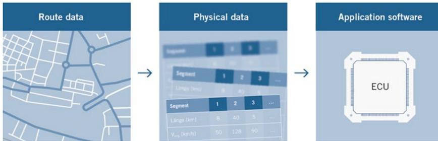
FIGURE 2 Signal flow and processing of navigation data (© Bosch)
